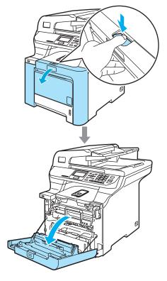
Hold the green handle of the drum unit. Lift the drum unit up and then pull it out until it stops.
